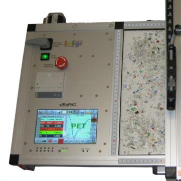
All measurement results can be grouped, listed and arranged as desired and printed out on the mini-plotter and/or at the connected PCprinter as a complete analysis report.
