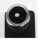
For plastic identification the unit is pressed on the surface of the sample and is measured by pressing the trigger button. Single measurements can be made as well as online (circular) measurements with a fixed trigger key.
