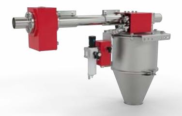
The **PLASTRON 05** K metal separator is placed directly on top of the plasticizing unit of injection moulding machines or an extruder. By means of a rotary cone mechanism and supporting compressed air system it reliably discharges contaminants, both when stationary material columns are lying flat and in free fall, with dust as well as with granules or ground material. It also carries complete feed units consisting of suction conveyor and mixer with high mechanical stability.
