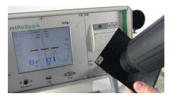
The identification of different plastic types for both spectrometers is the result of a trained pattern recognition with a specially developed neural network inside a database with several counterchecking. The result of the calculation is a list of the most probable polymer types identified within a probability between 0 and 100%. This comparison is necessary, since – contrary to metals – plastics have no norms and no standardizations!
