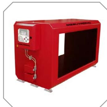
For particularly large dumping heights, such as grinding large tanks or foil bundles, it may be necessary to switch to closed tunnel detectors of the **METRON 05 C** series. These devices have a higher detection performance and can additionally be equipped with so-called »shielding extensions«. These reduce large-scale false alarms due to electromagnetic interference fields, which can greatly reduce the detection accuracy, in particular with passage heights exceeding 800 mm.
