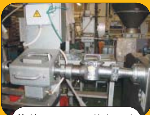
Metal detector on a support, used for the removal of non-magnetic particles.
