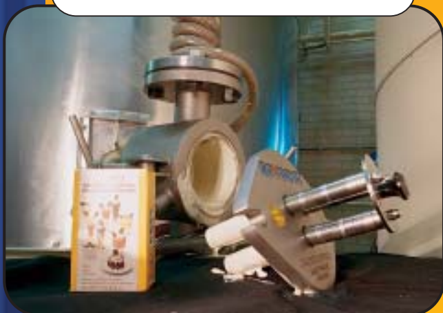
Magnetic filters used in chocolate production processes.
