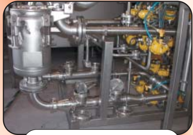
A double sanitary filter for deferrising ketchup
