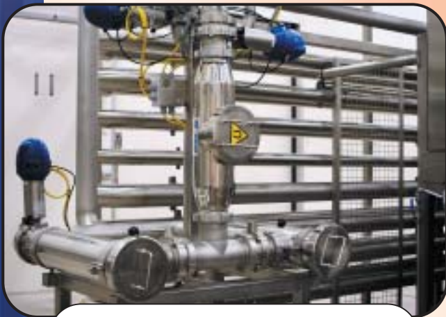
A sanitary filter for deferrising fruit juices.
