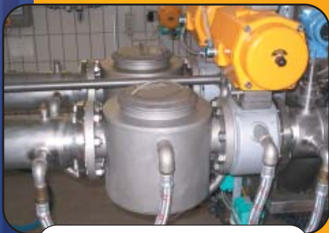
Magnetic filters used in chocolate production processes.
