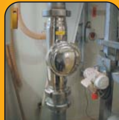
Magnetic filter in pneumatic transport pipeline removes Fe particles from milkpowder.
