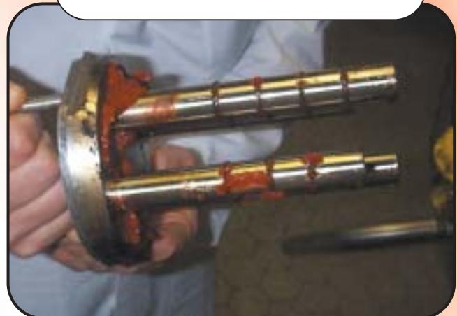
A double sanitary filter for deferrising ketchup
